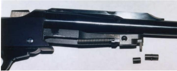
Remove the standard (short) forend retention pin. Slip the Hicks #1 Accurizer over the end of the forend hanger and insert the new (long) retention pin through the holes.
