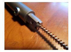
3. Apply oil to the edge of the chamber. Metal cutting oil is optimal, however any good gun oil will also work.
