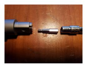
5. Locate the flat area on the ChamberMade. Insert the ChamberMade with the flat oriented towards the burr.
