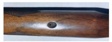
Drill the tuning access hole through the forend screw recess. Reattach your forend normally. Tune the Accurizer through the hole with an Allen® type hex wrench.
