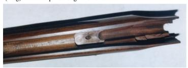
Use milling machine or Dremel with drum sander to inlet clearance for the Hicks #1 Accurizer in your forend.
