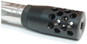
With the ports centered on top and the blank section centered on the bottom of the barrel, back out the Jam Nut until it butts up against the MS brake. Tighten the Jam Nut to lock the brake in place. To grip the MS brake while tightening, you can use a brass rod thru the ports or a strap wrench.
