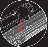
Hold the action firmly against the recoil lug secure with included action screws - tighten to 60 in-lb or an extra 1/4 turn past snug!
