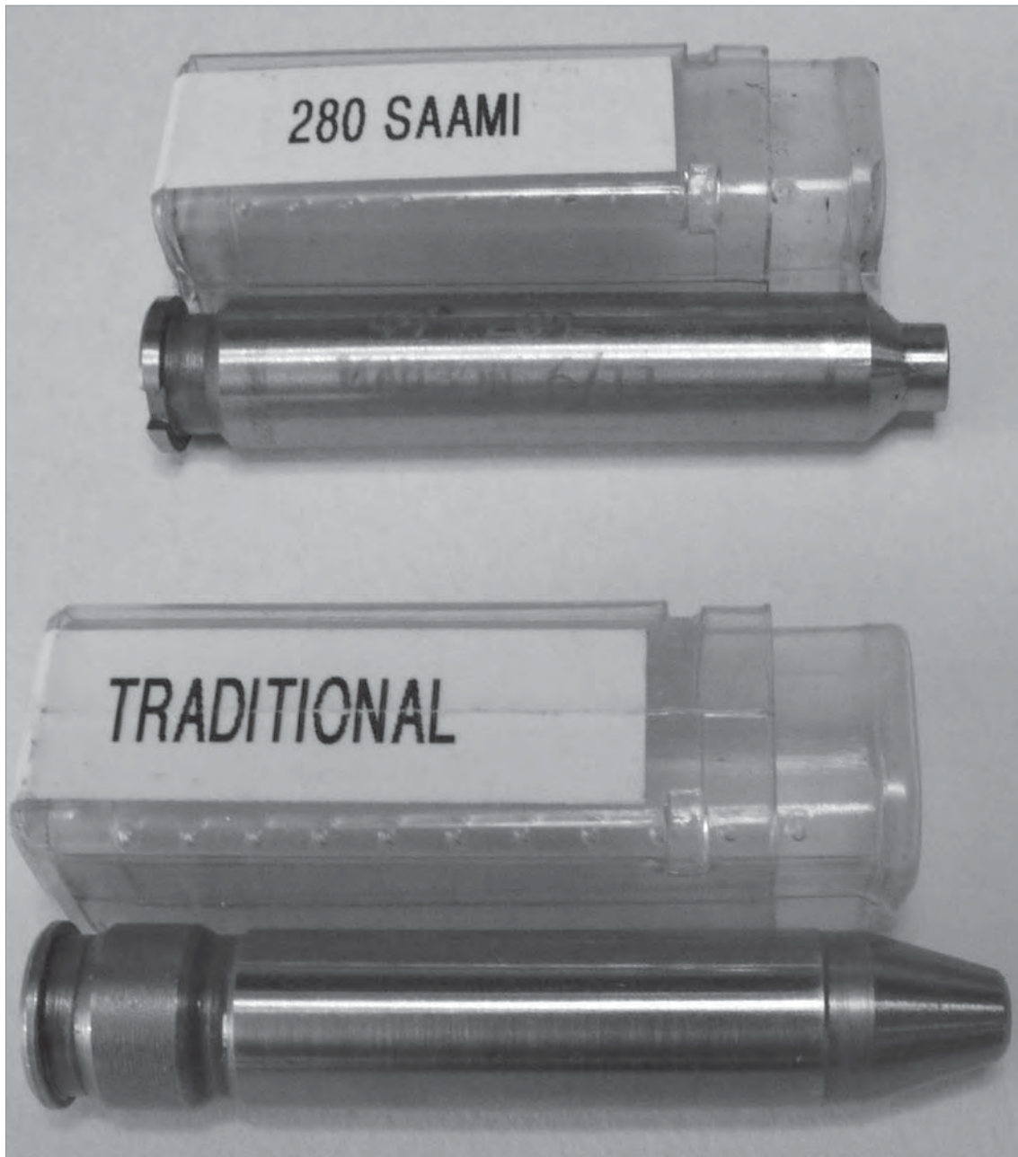
Comparing traditional gauges with true 40-degree gauges. They produce the same result.
