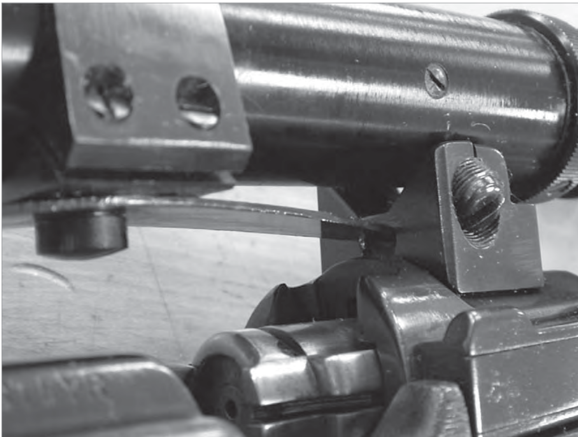
You can see the pivot screw in the bottom of the scope ring, the rear base, and the way that the attachment spring contacts the rear base. It's easy to see why these are commonly called "V- block" bases.
