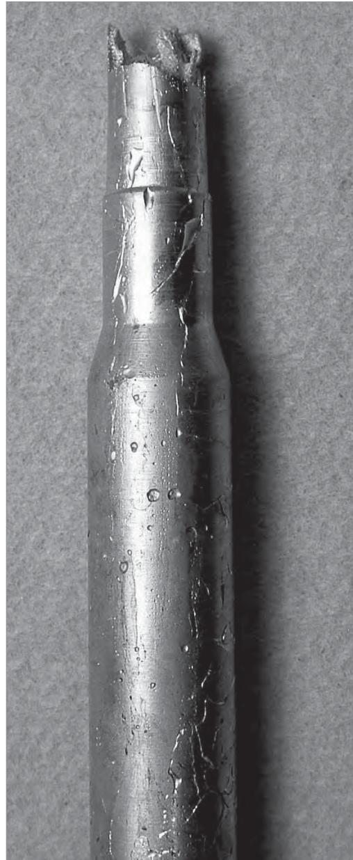
Chamber Cast with Cerrosafe, no visible damage to chamber. The photo is of the chamber cast from our test rifle after forcing the bolt closed. Note that there is no visible damage to the shoulder. However there is a relatively large surface area that would allow for the bolt to act like a jack and simply force the barrel forward in the receiver, thus changing the headspace.
