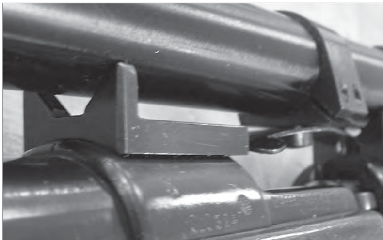
Note the front base and the “V” in which the scope rests. Just behind the base there is a tab of metal protruding just right for your right thumb to depress and release the spring to the side, allowing the scope to quick release.
