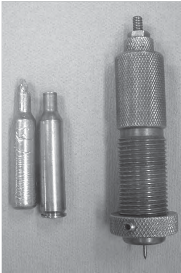
This is a die manufactured and provided by Ackley with one of his custom barrel jobs. Note the .228 Ackley size die, chamber cast and cold formed case (not yet fireformed).
