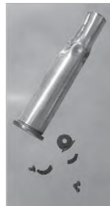
Primer failed with excessive headspace of .046 inches.
