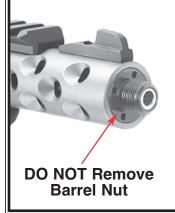
When removing the muzzle cap, a barrel nut is behind the cap and washer. This nut is used to lock the barrel in place. This nut should never be loosened, removed or tampered with. This nut is epoxied and torqued in place at the factory. This nut is meant to remain in place and should not be removed under any circumstance. Failure to follow this warning will cause permanent damage to your firearm and will not be warranted or repaired by Customer Service.
