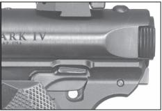
Figure 6. Safety in the "on" or "safe" position. Safety is <u>all the way up and the white dot is visible.</u>
